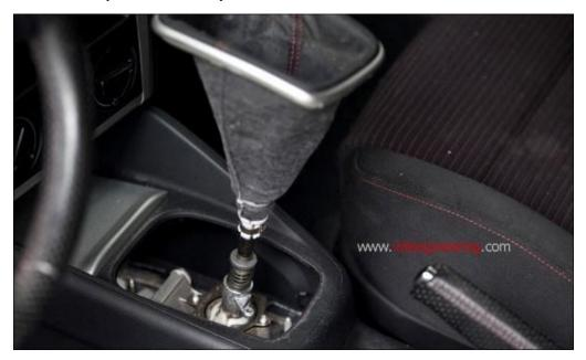
On the side of the shifter you will see two holes. Get your 4mm allen key and slide it into the two holes. This will center the shifter. If you find there to be resistance while trying to align the holes on the shifter, do not force the shifter. The problem is that the shift cables are binding on the shift end links. You simply need to free the binding that is occurring.
