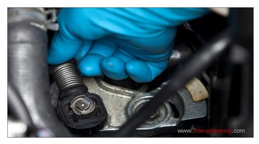
Place the blade of the small flat tip screwdriver under the center tab of the silver retaining tabs that keeps the end links mounted to the pendulum. Carefully lift the center of the tabs up and remove. Do not lose these tabs. Follow this procedure to completely remove both end links from their mounting points.
