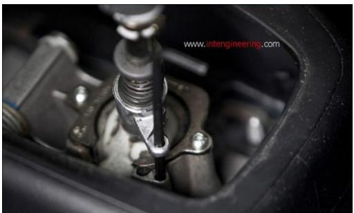
Once the shifter has been centered, go to engine bay. Release the lock ring by rotating the ring in the clockwise direction so that the shift end link is locked back onto the shift rod. Once the end links are locked back on the the shift rods, pull the pendulum lock pin back out.
