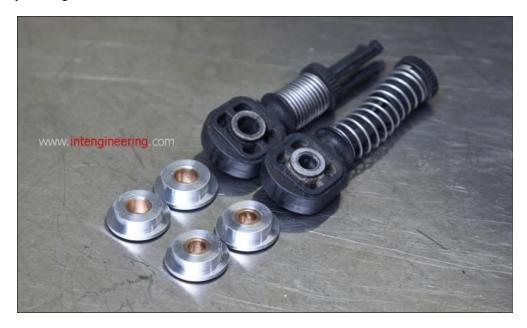
There is a rubber bushing connected in each corner using plastic tabs. Firmly press down in each corner with your small blade screwdriver until you hear a snapping sound. At that point the retainers should be broke and the rubber portion should be ready to remove. Follow this step for each end.
