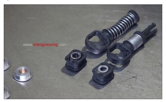
Assemble each of the end links by firmly pressing each IE solid bushing into the area where the original bushing was housed. Remember that the centers of the bushings are different sized, so make sure as to not mix the corresponding sizes up. Both solid bushings can be installed into the end links in this.
