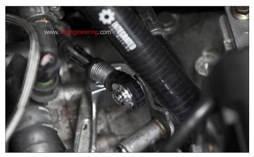
Now it is time to align you shifter inside of the vehicle. Locate the locking pin below the shift pendulum. While pressing down on the shift pendulum, push the locking pin into the transmission. You may have to release the pressure on the pendulum in order to allow the locking pin to slide into place. Once you feel the pin slide into place, the shift pendulum will be locked in place.
