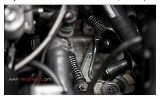
Grab the base of the end link that is connected to the shift cable and slide the lock ring forward compressing the spring. Once the spring has been compressed, rotate the lock ring in the counterclockwise direction and release. Complete this step for both end.
